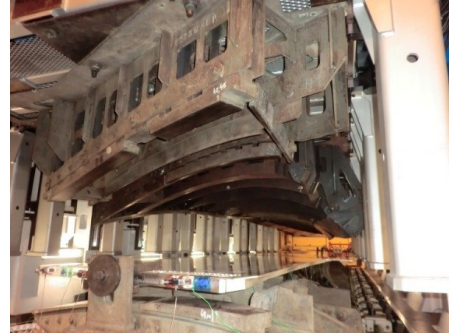
Figure 5. View of the panel just before cold forming.
