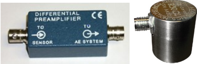
Figure 6. In-line miniature preamplifier (8.26cm x 2.87cm x 2.22cm, 54 grams) and R50a sensor (19 x 20 mm, 32 grams).
