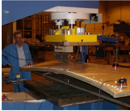
Figure 2: Example of “manual” cold forming with single punch press.
