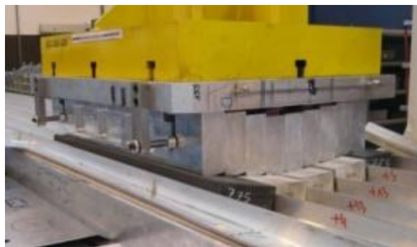
Figure 3: Example of “manual” multiple punches shot cold forming.
