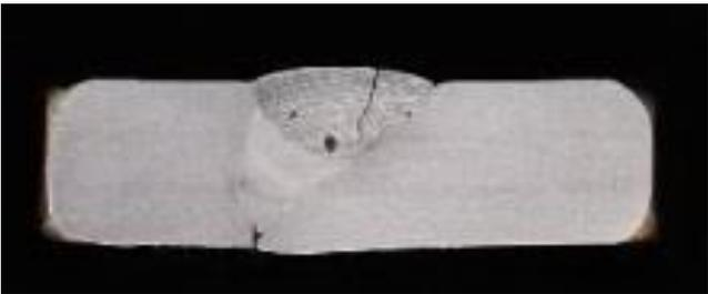
**Fig.5.** The general view of the defects: incomplete welding, crack and pore
