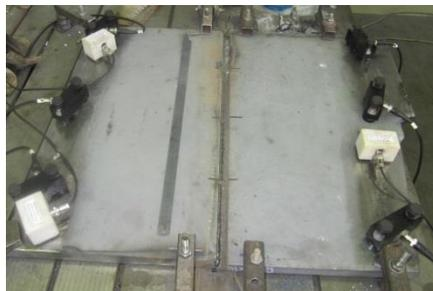
**Fig.1.** Location of the AE sensors on the sample of a butt welding junction
