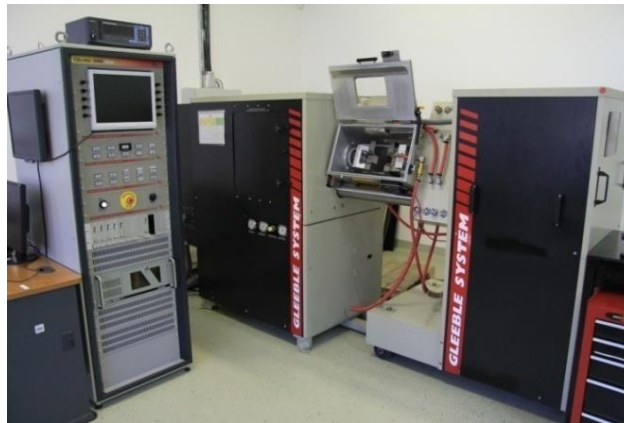
Pic. 1. The Gleeble 3800 thermomechanical simulator
