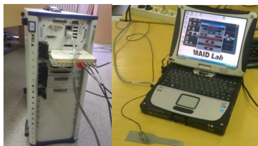
Pic. 2. The measurement system with the NI PXIe embedded computer and a personal computer for control purposes.
