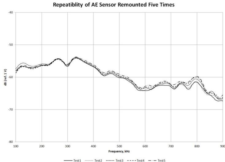
**Fig. 2.** Repeatability of measurements tested and remounted using 1/4-20 UNF 2A SHCS
