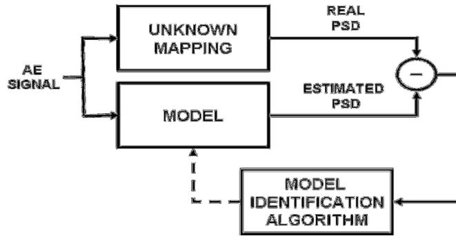
Fig. 12. Conceptual layout of POWdER Algorithm
