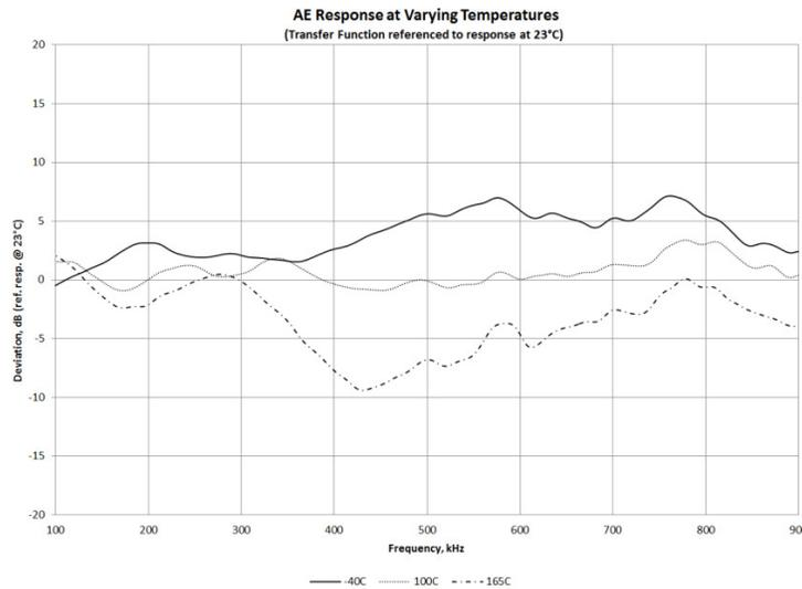
**Fig. 4.** Temperature response curves at various temperatures, normalized by the response at  $23^{\circ}\text{C}$
