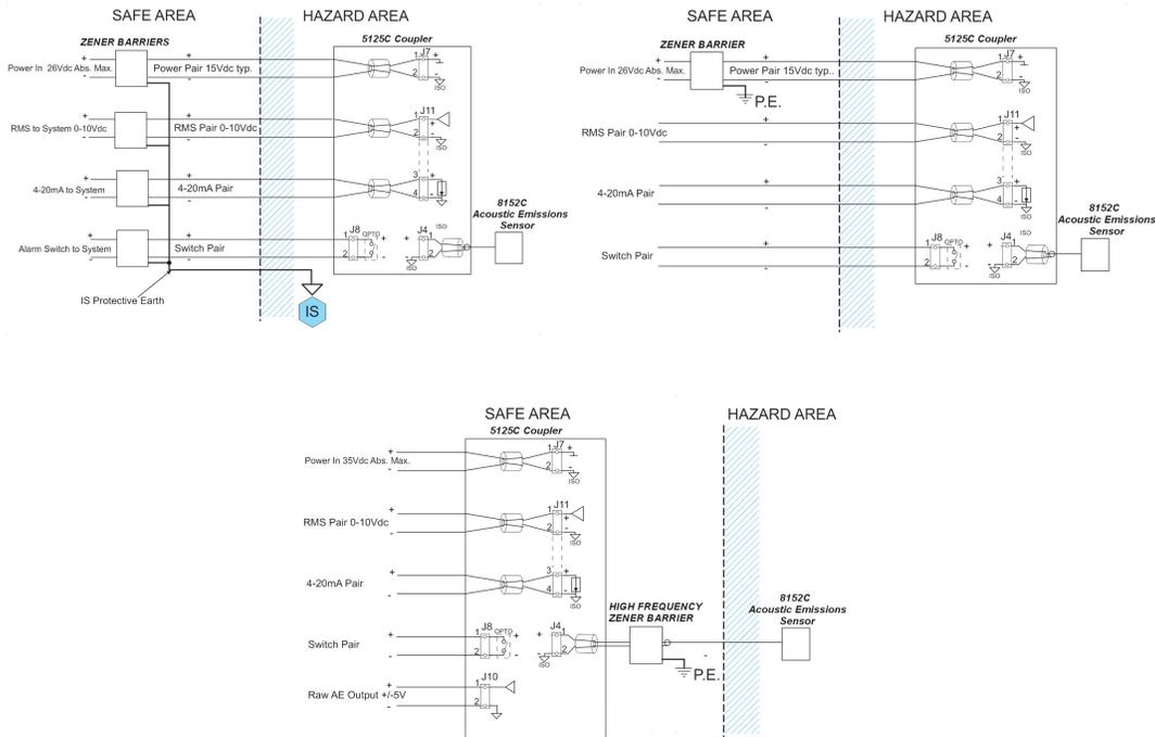
**Fig. 10a.** ATEX/CSA Hazardous Area Installation for Zone 0 (upper left)
