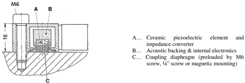
**Fig. 1.** Acoustic Emission sensor type 8152C, Cross Section
