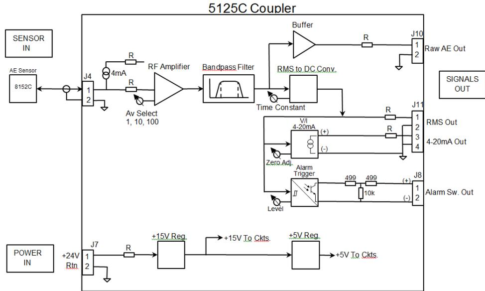
**Fig.7.** AE Measuring Chain (Block Diagram)
