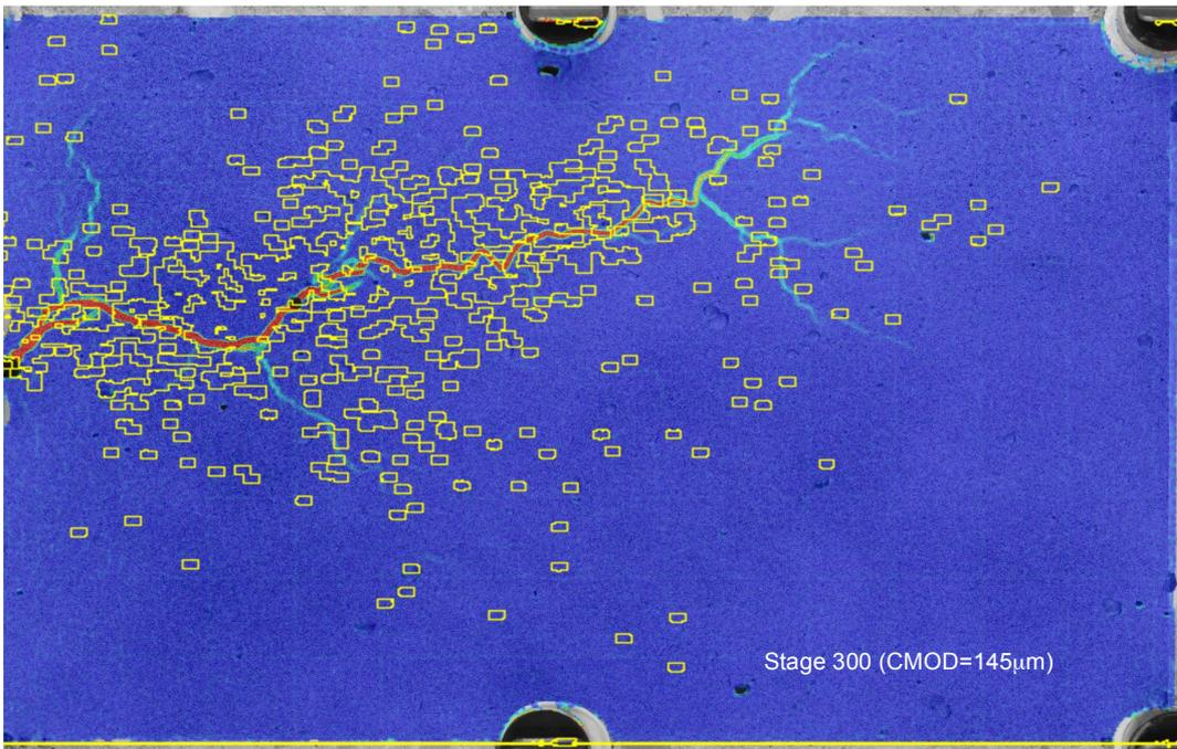
**Figure 5.** Overlay of DIC measurements and AE signals obtained up to CMOD = 145µm
