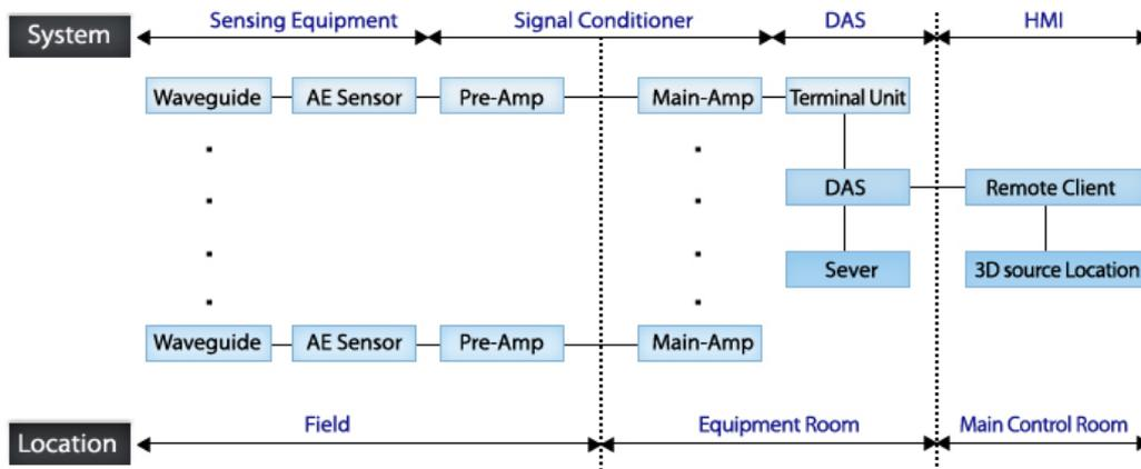
Fig. 2. System configuration of BTLD
