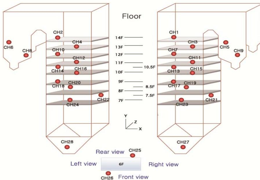
**Fig. 4.** Mirror type sensor location map for sensors (28 channels): (a) left view; and (b) right view.
