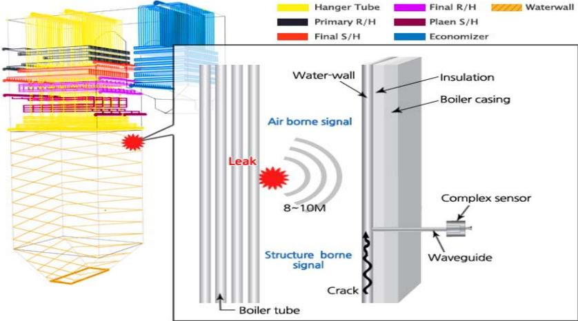
**Fig. 1.** Tube Leak Detection Method
