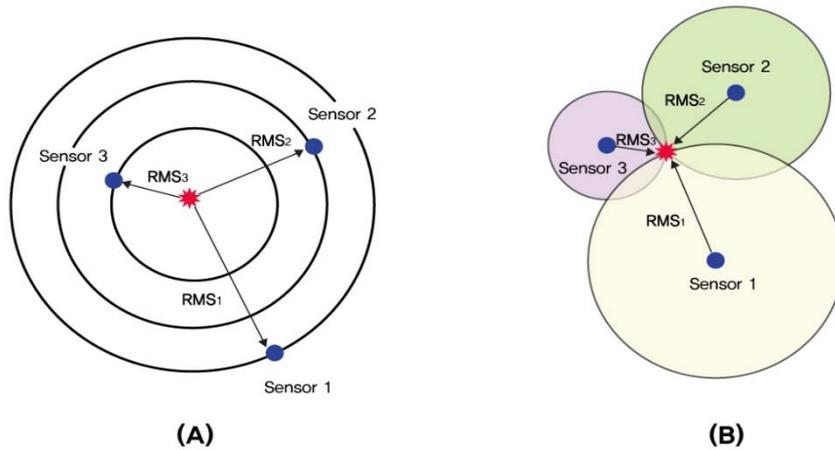
**Fig. 3.** Estimating the position of leakage in 2D by means of sensor RMS magnitude ratio [20]: (a) Signal propagation from actual leakage point to sensors; and (b) Estimated leakage propagation by using sensors.
