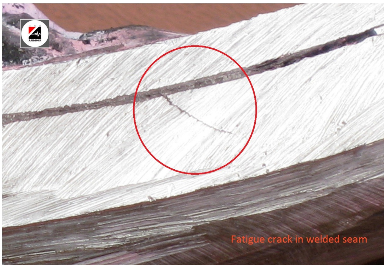
Fig. 5. The fatigue crack which has been found out ISHM «Ресурс-2000» in a welded seam of the refinery pipeline.
