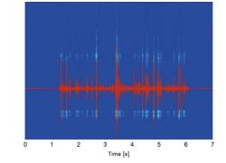
Each Burst excites an individual (based on sensor) frequency spectrum
