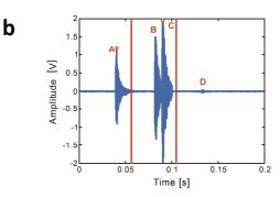
Analyzing an AE Signal vertically rather than horizontal leads to an exact burst maximum
