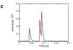
Because of the short rising time of an AE Burst it is possible to detect them using a slope indicator
