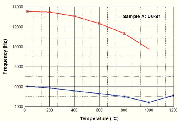
**Fig.9** Specimen degradation induced predominant frequency shift caused by elevated temperature. The hammer hit the specimen in the longitudinal centre line direction, perpendicularly to the signal propagation direction. The upper curve shows the trend of frequency  $f_2$ , the bottom curve shows the trend of frequency  $f_1$ .
