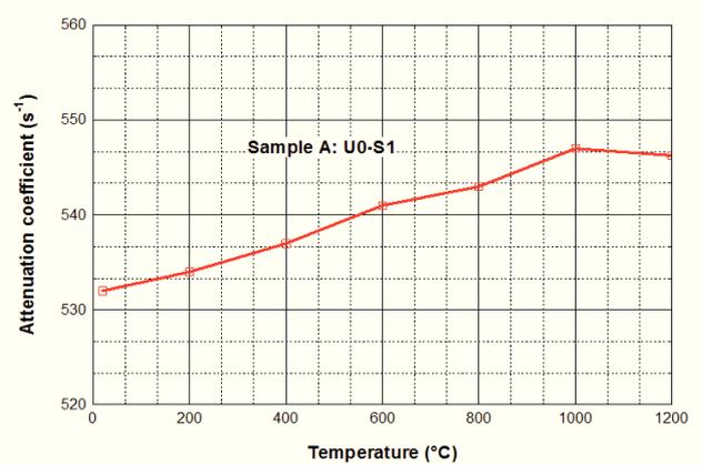
**Fig.10** Specimen degradation induced damping coefficient change caused by elevated temperature. The hammer hit the specimen in the longitudinal centre line direction, the sensor was placed in the middle of the specimen face, perpendicularly to the signal propagation direction.
