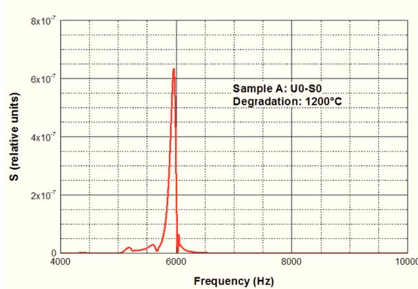
**Fig. 5** Frequency spectrum for the sensor placed at the end of the joist and the hammer blow at the opposite end in the longitudinal centre line direction. The specimen was stressed by an elevated temperature of 1200°C.
