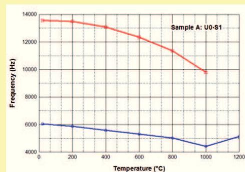
Fig.5 Specimen degradation induced predominant frequency shift caused by elevated temperature. The hammer hit the specimen in the longitudinal centre line direction, perpendicularly to the signal propagation direction. The upper curve shows the trend of frequency  $f_2$ , the bottom curve shows the trend of frequency  $f_1$ .
