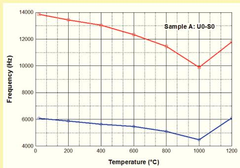
Fig.3 Specimen degradation induced predominant frequency shift caused by elevated temperature. The red curve shows the trend of frequency  $f_2$ , the blue curve shows the trend of frequency  $f_1$ .
