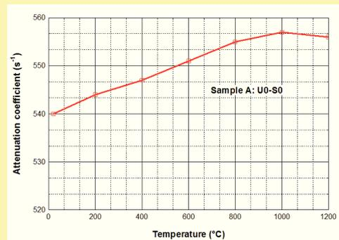
Fig.4 Degradation induced damping coefficient change caused by elevated temperature.
