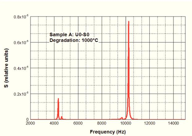
**Fig. 3** Frequency spectrum for the sensor placed at the end of the joist and the hammer blow at the opposite end in the longitudinal centre line direction. The specimen was stressed by an elevated temperature of 1000°C.
