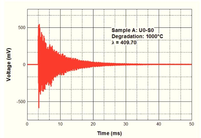
**Fig. 4** Recorded signal time response for the specimen, which has been stressed by an elevated temperature of 1000°C.
