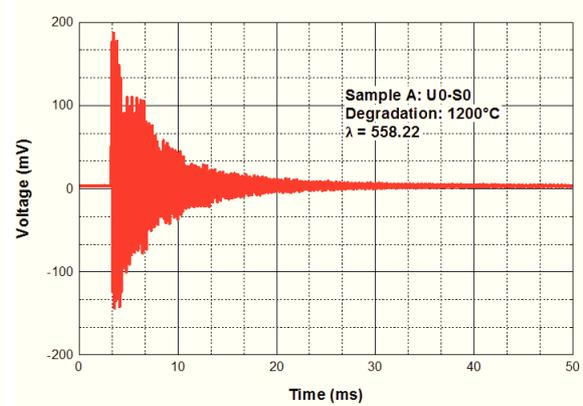
**Fig. 6** Recorded signal time response for the specimen, which has been stressed by an elevated temperature of 1200°C.
