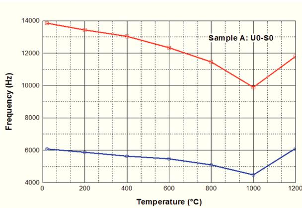
**Fig. 7** Specimen degradation induced predominant frequency shift caused by elevated temperature. The red curve shows the trend of frequency  $f_2$ , the blue curve shows the trend of frequency  $f_1$ .
