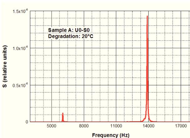
**Fig. 1** Frequency spectrum for the sensor placed at the end of the joist and the hammer blow at the opposite end in the longitudinal centre line direction. The specimen was not stressed by elevated temperature. Reference specimen. Temperature,  $20^\circ\text{C}$ .
