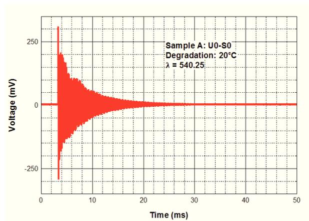
**Fig. 2** Recorded signal time response for the specimen, which has not been stressed by elevated temperature. Temperature,  $20^\circ\text{C}$ .
