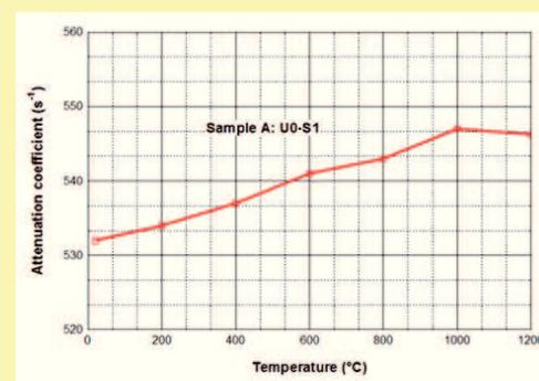
Fig.6 Specimen degradation induced damping coefficient change caused by elevated temperature. The hammer hit the specimen in the longitudinal centre line direction, the sensor was placed in the middle of the specimen face, perpendicularly to the signal propagation direction.
