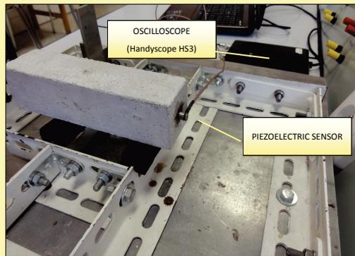
FIG.1, FIG. 2 IN ORDER TO GENERATE THE ACOUSTIC SIGNAL, A HAMMER OF 12 G MASS, ORIGINALLY SUSPENDED FROM A HANGER, WAS RELEASED TO FALL DOWN ON THE SPECIMEN FROM A HEIGHT OF 4 CM. THE RESPONSE WAS PICKED UP BY AN MIDI TYPE PIEZOELECTRIC SENSOR, WHOSE OUTPUT VOLTAGE WAS FED INTO A TIEPIE ENGINEERING HANDYSCOPE HS3, WHICH IS A TWO-CHANNEL, DIGITAL, 16 BITS OSCILLOSCOPE. SUBSEQUENTLY, A SPECIAL SMOOTHING ALGORITHM WAS USED TO DETERMINE DOMINANT FREQUENCIES FOR EACH OF THE OUTPUT SIGNALS.
