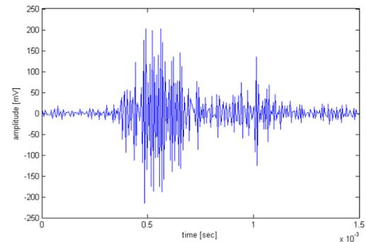
**Fig. 8** Results with broad band-sensitive sensor followed by digital band pass filtering (85 – 100kHz)
