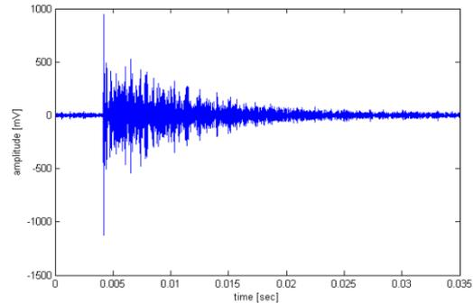
**Fig. 10** Broad band-sensitive sensor followed by digital band pass filtering (85 – 100 kHz)
