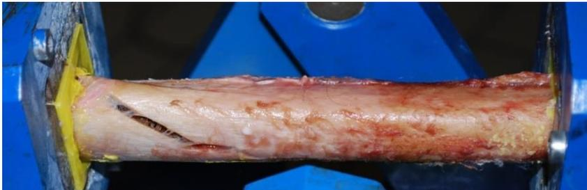
**Fig. 13** Fracture image of osteoporotically altered human femur subjected to bending- torsional load
