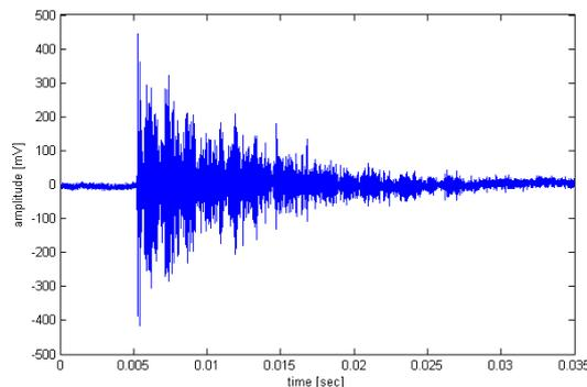
**Fig. 4** Discrete emission due to crack formation (resonant sensor 100kHz)
