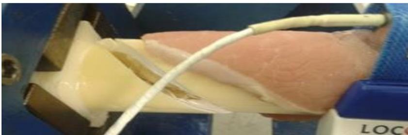
**Fig. 15** Fracture image of artificial bone subjected to bending-torsional load. [4]
