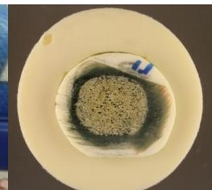
**Fig. 16** View on the structure of an artificial bone showing a compact part at the outer zone and a more or less porous material in center parts. [4]
