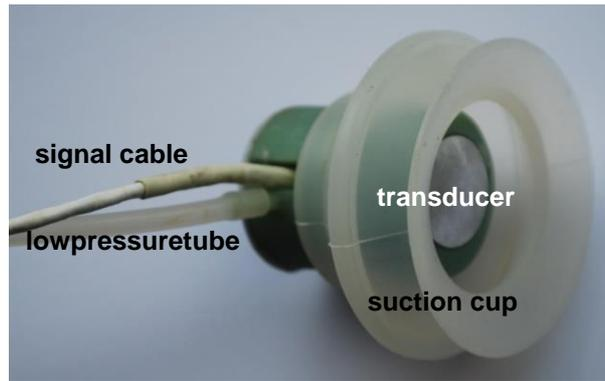
**Fig. 1** Sensor with suction cup for a well defined sensor attachment.
