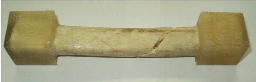
**Fig. 11** Fracture image of healthy human femur subjected to bending-torsional load [5]
