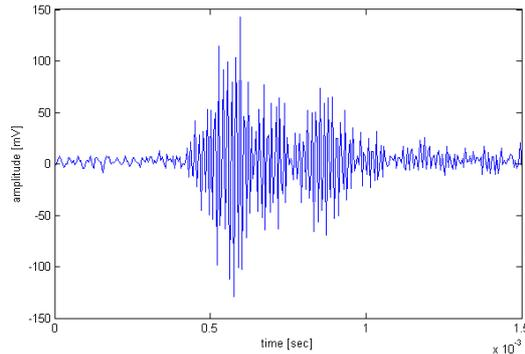
**Fig. 3** Continuous acoustic emission associated with a cartilage lesion in a human knee joint (resonant sensor: 100kHz)
