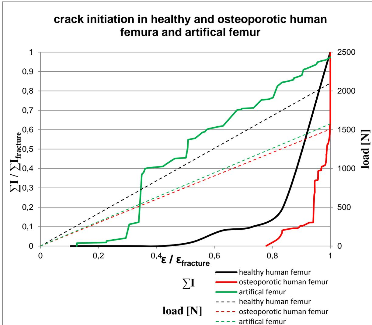
**Fig. 17** Crack formation in donated healthy and osteoporotically altered human femora and in artificial femora. [4, 5]
