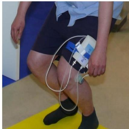
**Fig. 2** Proband in action equipped with the measuring system (emission sensor coupled to lateral femoral condyle; measuring device including the position sensor coupled to the proximal thigh)
