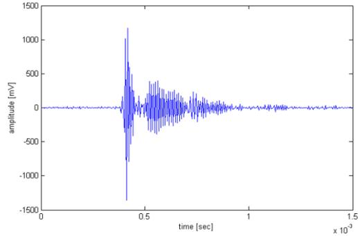
**Fig. 6** Results with broad band-sensitive sensor followed by digital band pass filtering (85 kHz - 100kHz)
