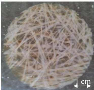
Fig. 3. Picture of consequences of the corrosion on GFRP
