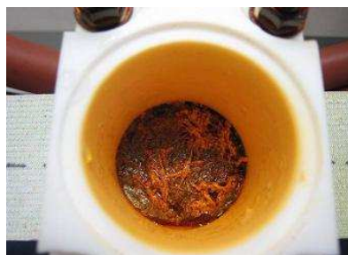
Fig. 11. GFRP specimen after corrosion test with bromine
