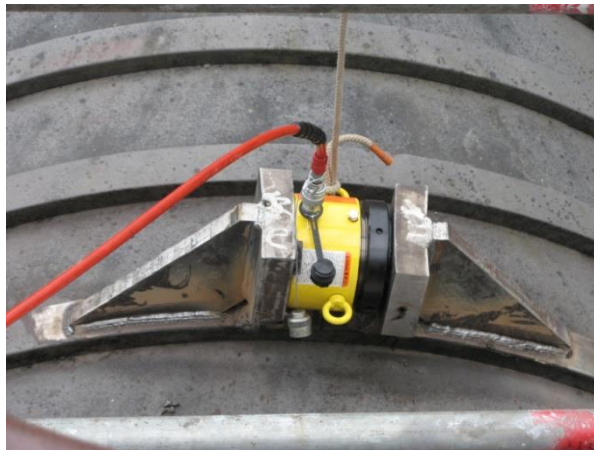
Picture 2: Rupture test of a forged hoop–Hydraulic System
