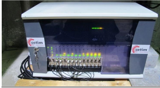
Picture 12: Vallen Acquisition System + Inverter + PC
