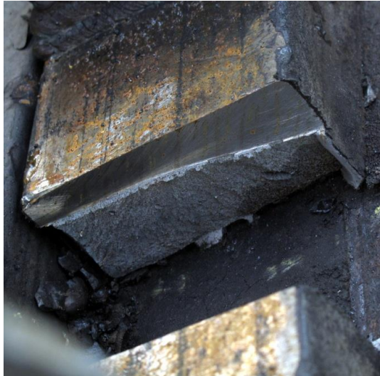
Picture 3: Rupture test of a forged hoop– Fracture Surface
