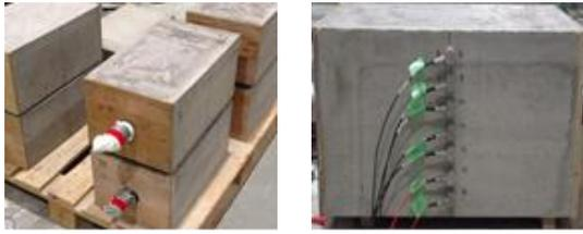
**Fig. 11.** The arrangement of AE sensors
