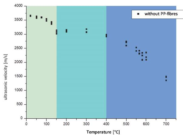
**Pic 4:** Relation between temperature and the ultrasonic velocity inside the furnace [3].
