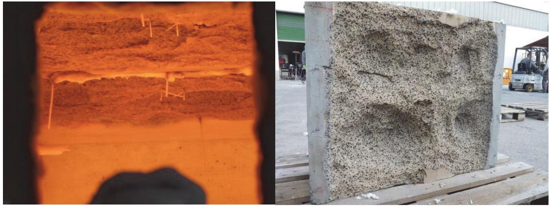
**Pic. 2:** View to the specimen inside the furnace with concrete damage because of spalling (left) and a damaged specimen after the experiment (right).
