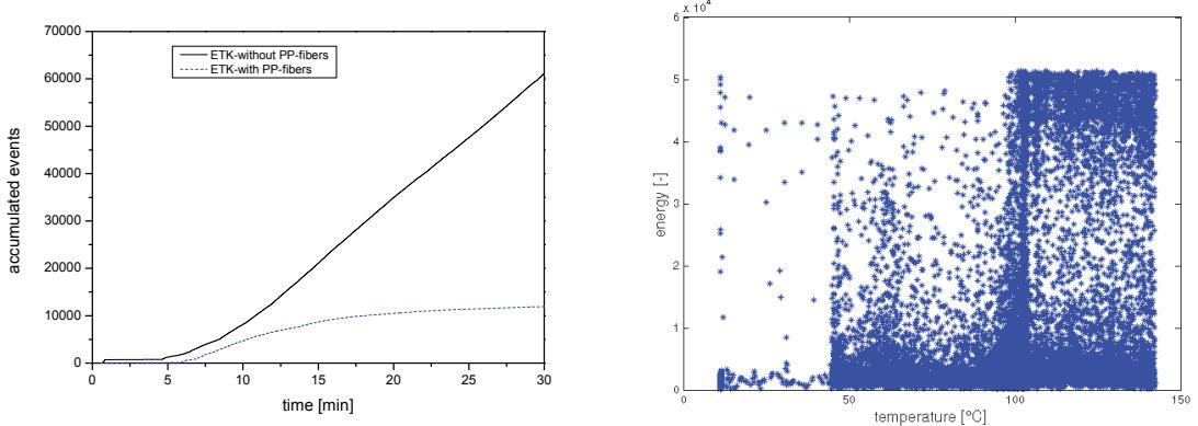
**Pic. 3:** Acoustic emission activity of specimen with and without PP-fibres tested according to the modified ZTV-Ing standard (left). Occurrence of AE events and their signal-energy plotted over temperature (right) [8].
