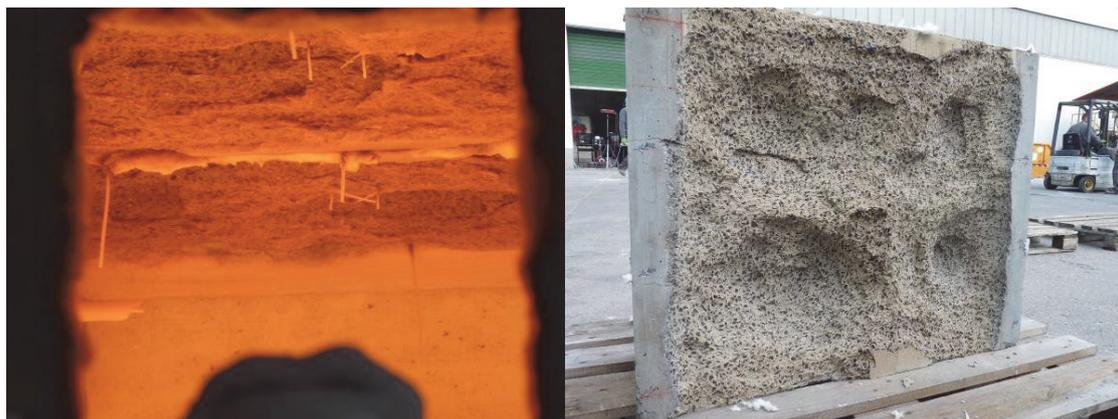
**Fig. 2:** View to the specimen inside the furnace with concrete damage because of spalling (left) and a damaged specimen after the experiment (right).
