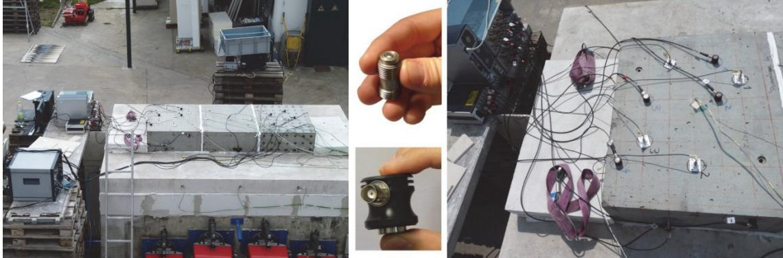
**Pic 1:** Specimen on top of the furnace with the connected measurement systems (left) Different types of sensors (middle) and their application on the surface of the specimen (right).
