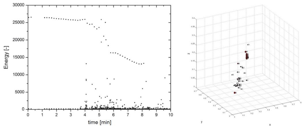
**Pic 6:** Signal-energy over time of an experiment with an synthetic AE-source (left) and a 3D-localization of the ultra-sonic signals (right) [9].
