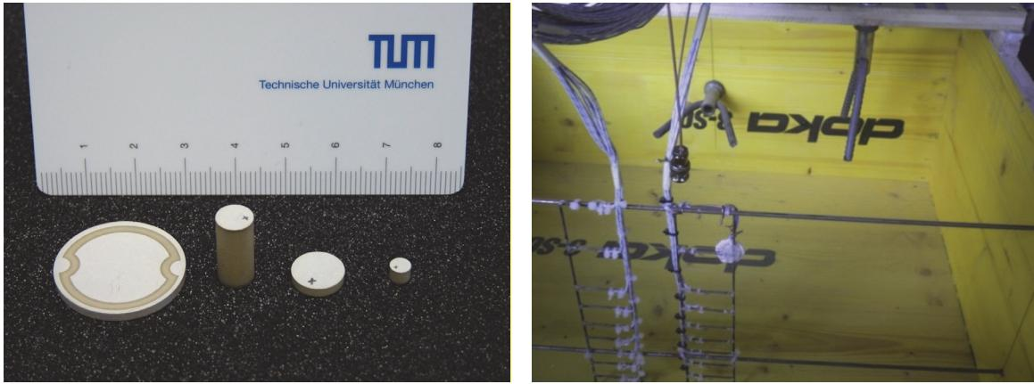
**Pic 5:** Different piezo-ceramics to prepare synthetic ultrasonic sources(left) [4] and the application of synthetic sources in the concrete formwork (right) [9].
