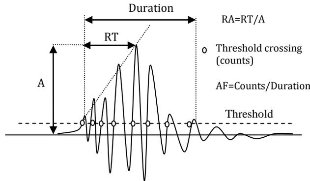
**Pic 1.** Typical AE signal and its main characteristics.
