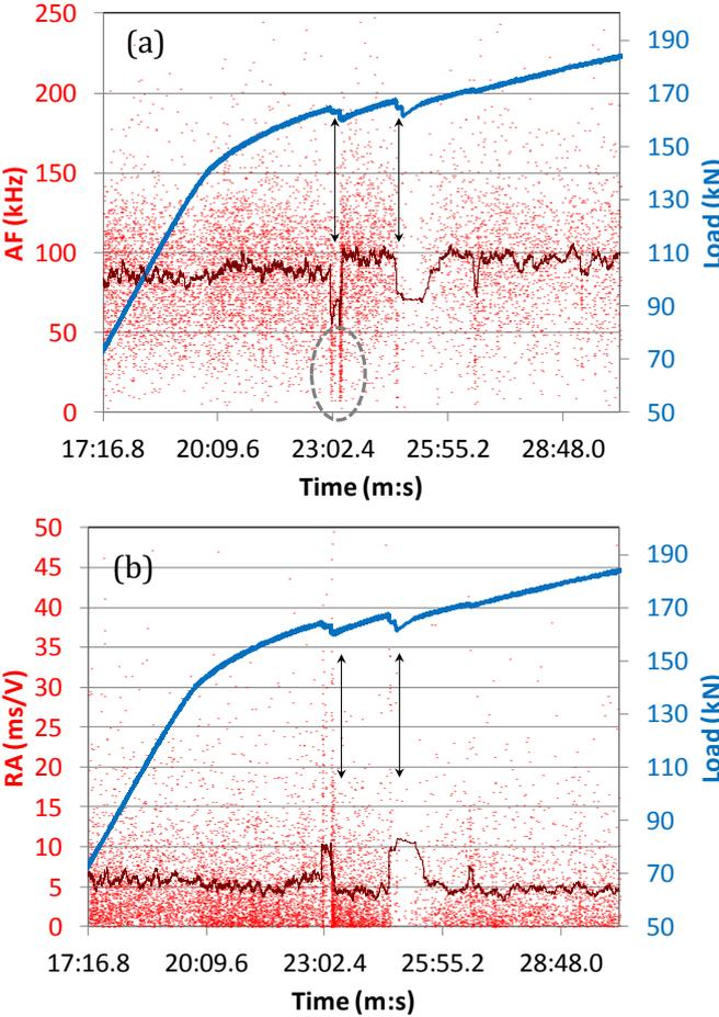
**Pic. 3.** Load history along with (a) AF, (b) RA value of the CFRP reinforced beam. The line is the moving average of 100 points.
