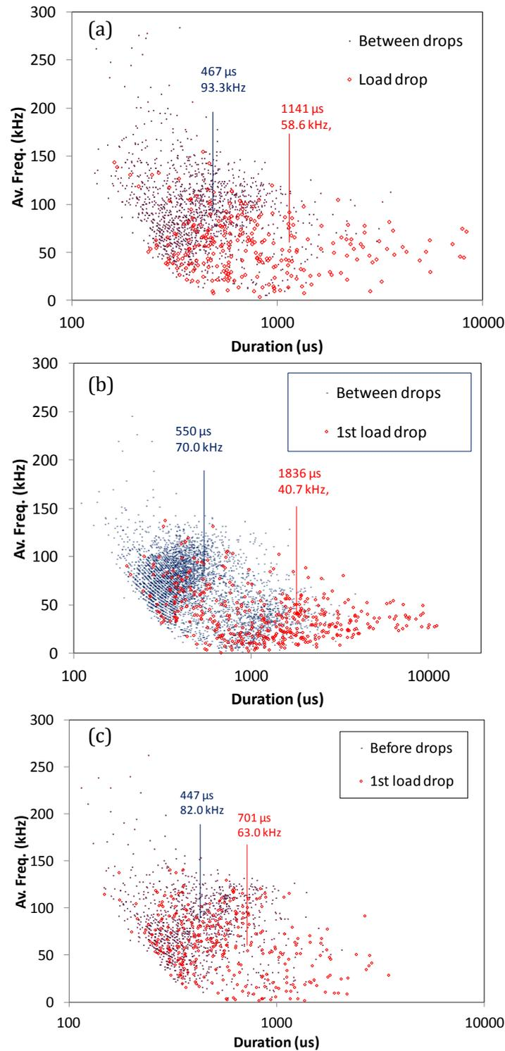
**Pic. 4.** AF-RA correlation plots for (a) CFRP beam, (b) TRC reinforced beam, (c) TRC reinforced pre-cracked beam.
