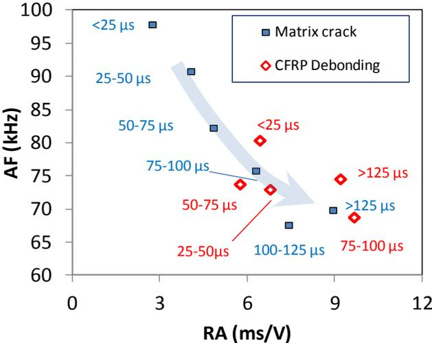
Pic. 5. Correlation plot of AF vs. RA for AE hits from CFRP debonding and concrete cracking.
