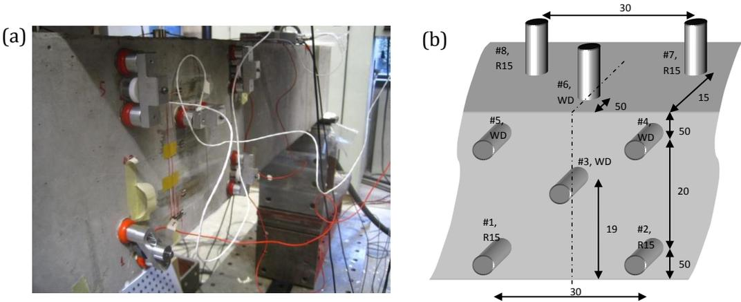
**Pic. 2.** (a) Photograph and (b) schematic representation of the experimental AE setup.
