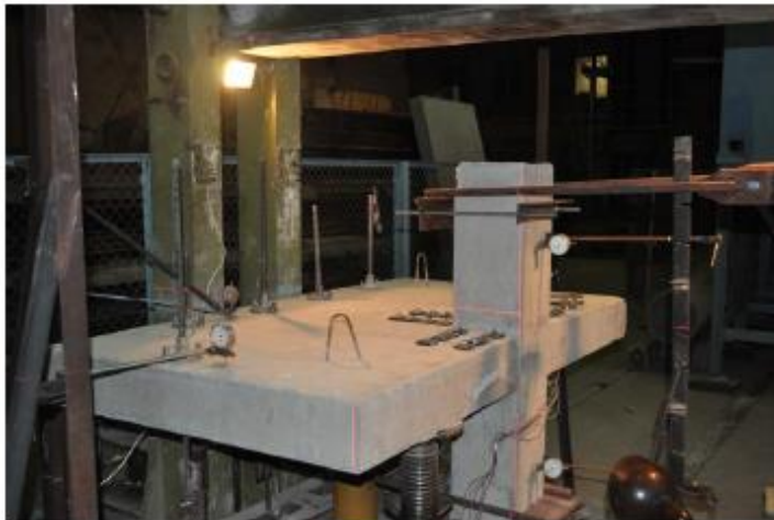
Pic. 2. Experimental sample made as a section of a floor slab and columns.
